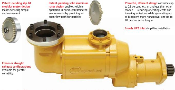
Patent-pending, fully supported high-speed rotor extends bearing life by minimizing deflection and ensuring concentric running Aerodynamic speedlimited design and steel containment ring provide fail-safe reliability Integral slip clutch design eliminates need for soft-start valve or other controls, reducing shock-loading and ensuring better protection of unit **Pre-engaged front end** delivers time-proven durability
